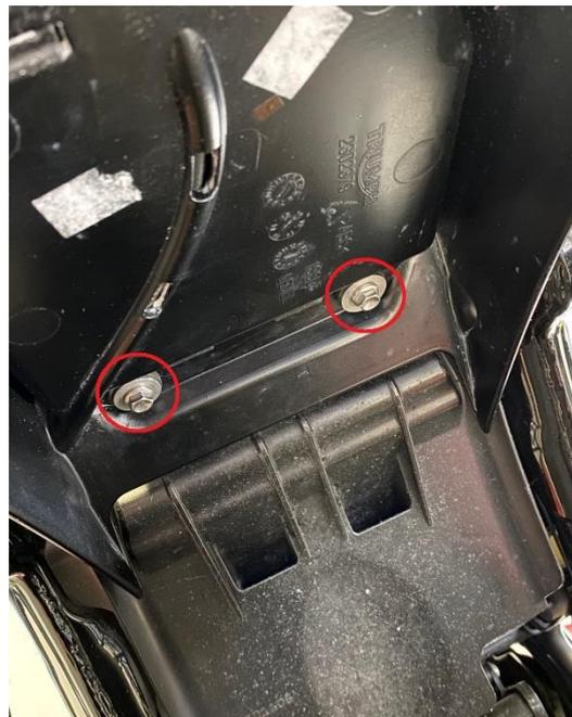
9. Unclip the retaining plate from the ECU, remove the ECU and hang it to the side.
