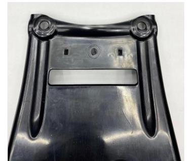
Trim the interior trim as shown in the pictures. Roughly cut with a side cutter and grind into shape afterwards.
