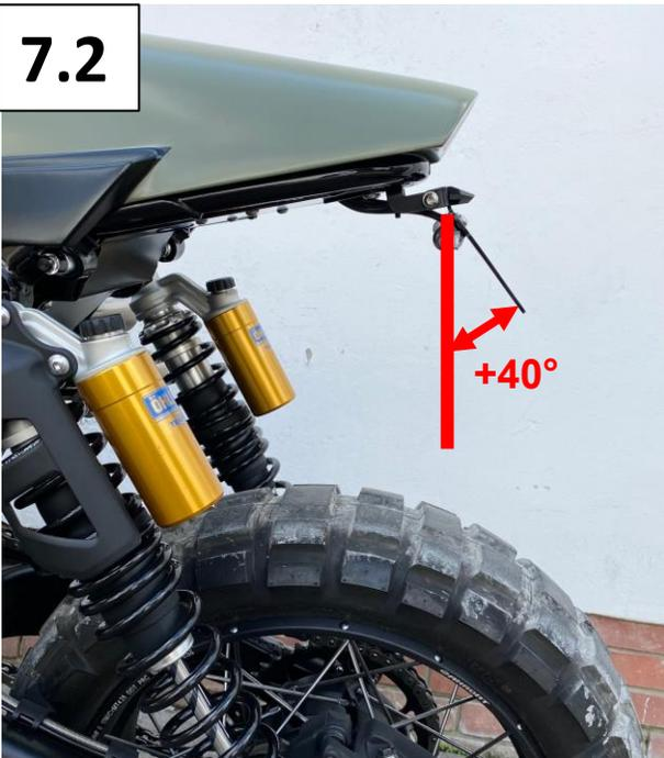
Adjust the license plate angle and tighten the screw connection WELL!
